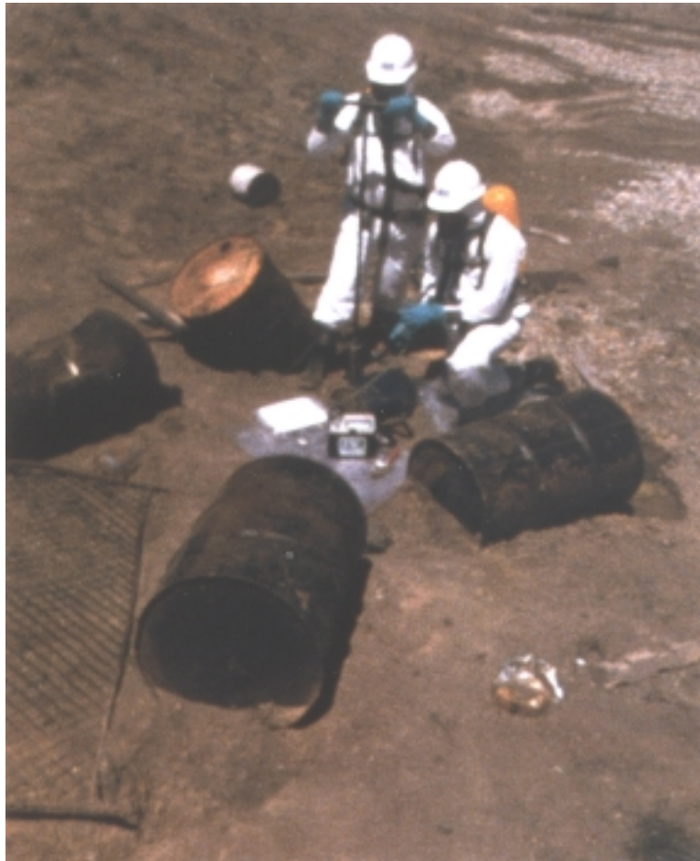
Figure B.8 – Soil sampling for radioactive contamination.
