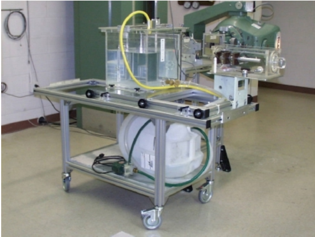
Figure A.7.1a -- Water phantom set up for absorbed dose to water measurements. (Courtesy of K&S Associates)
